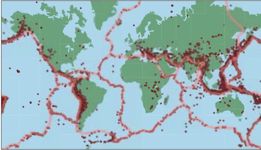
Figure 2. Although most seismic activity takes place at the boundaries between tectonic plates ( pink lines ), earthquakes of substantial size sometimes strike well within plate interiors. The red dots show the locations of earthquakes with magnitudes of 5.5 or more that have taken place since 1973. (Plate boundaries are derived largely from Rice University's Discovering Plate Boundaries Project; earthquake epicenters are from the catalog of the U.S. Geological Survey's National Earthquake Information Center.)
