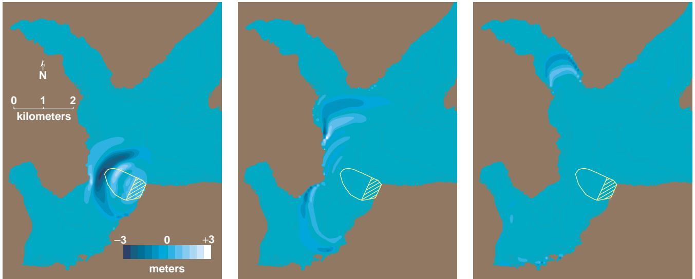
Figure 8. Numerical modeling illuminates how a single failure at the lake margin ( hatched area ) and its resulting slump deposit ( yellow outline ), one of several known to have been caused by the 470 B.C. earthquake, would give rise to a tsunami-like disturbance on the surface. Unlike normal, wind-driven waves, the undulation in water level has an enormous wavelength, nearly a kilometer. It also has an enormous size: One minute after the margin of the lake gives way in the simulation, the peak-to-trough amplitude of the wave is almost 6 meters ( left ). The wave propagates rapidly away from the site of initiation, traveling about 2 kilometers into two of the arms of the lake during the next minute ( center )—that is, with the speed of highway traffic. Three minutes after the simulated initiation, most of the disturbance is limited to the northwestern limb of the lake ( right ). In actuality, the multiple slope failures at different points around the lake generated several waves of this type, making for what must have been a highly complex pattern on the surface as the various waves interfered.
