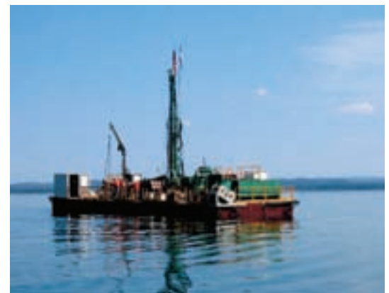
Between Feb 3 and March 11, 2006, drilling was conducted by DOSECC on Lake Petén Itzá using the Global Lake Drilling (GLAD800) drill rig, mounted on the "superbarge" R/V Kerry Kels. (Photo: PISDP)
